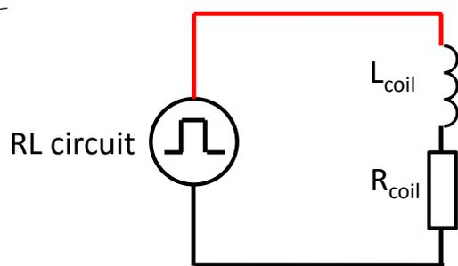
$$i_{RLcoil}(t) = \frac{U}{R_{coil}} \left( 1 - \exp\left(-\frac{t}{\tau}\right) \right)$$
