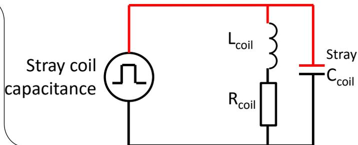
$$Z_{RLCcoil} = \frac{(R_{coil}^2 + L_{coil}^2 \omega^2) [R_{coil} - j\omega(C_{stray} R_{coil}^2 + C_{stray} L_{coil}^2 \omega^2 - L_{coil})]}{R_{coil}^2 + \omega^2 (C_{stray} R_{coil}^2 + C_{stray} L_{coil}^2 \omega^2 - L_{coil})^2}$$
