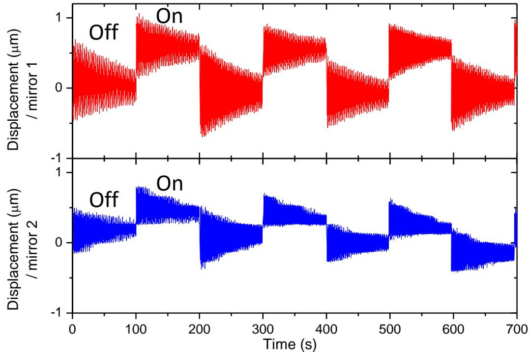
A damping of pendulum is visible after an On or Off sequence.
