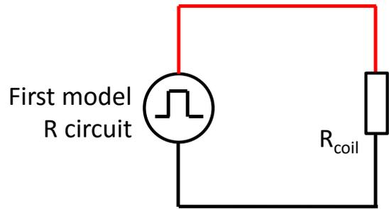
$$i_{Rcoil}(t) = \frac{U(t)}{R_{coil}}$$
